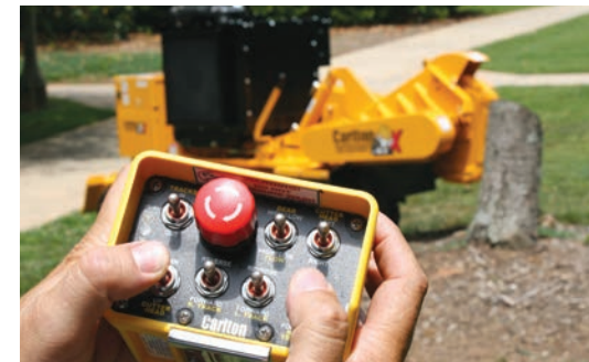
Carlton's wireless remote distances the operator from dirt, dust, and noise while increasing their visibility of the area being worked – reducing fatigue
