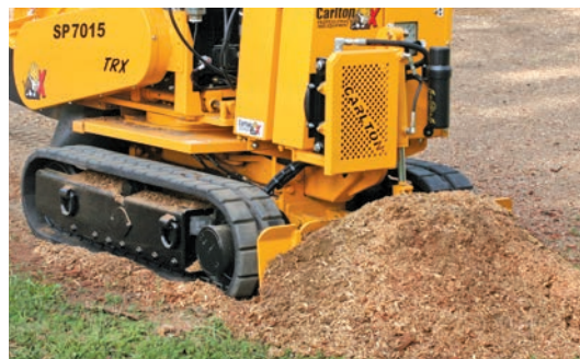
Optional Hydraulically Controlled Scrape Blade provides ability to spread or move chip piles – making quick work of clean up.
