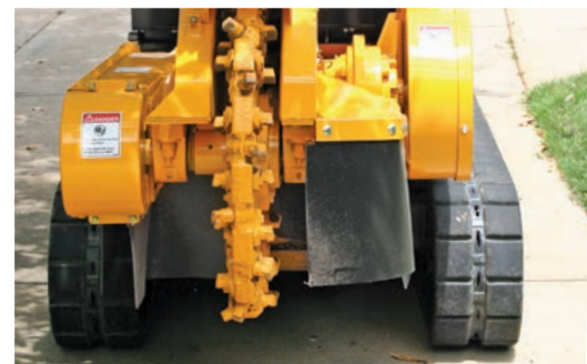
Extendable and retractable tracks hydraulically contract from 48- to 35- inches allowing access to tight working conditions. Turf friendly rubber tracks deliver maximum climbing power and minimal lawn disruption.
