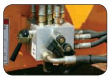
Integrated Single Manifold Hydraulic System simplifies the system reducing the number of hoses needed and reduces leak points.
