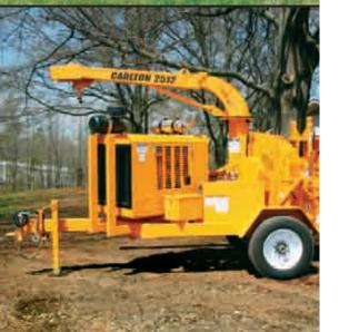
**8000 lb. Dexter Torflex Axle** with electric brakes makes Carlton 12" Chippers tow great. A 9000 lb. axle is used on the HD models.
