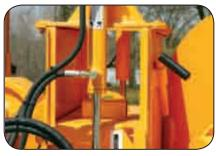
**Dual Lift Cylinders** provide crushing power when necessary and allow easy access to the anvil. Mounting these dual lift cylinders low on the sides allows for a full 360° discharge chute rotation.
