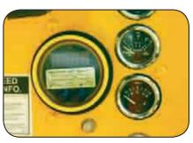
**Digitally Controlled Reversing Autofeed Plus** monitors engine rpm and adjusts the feed automatically. This system has the ability to start, stop, and reverse the feed of material into the chipper based on parameters set by the operator.
