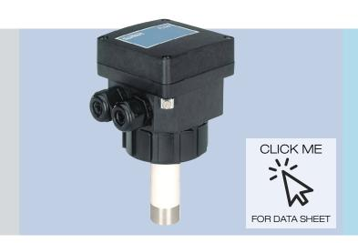
The insertion magmeter constructed from a PVDF finger and high quality blind electronic module. Perfect for contaminated or aggressive fluids it has both 4-20 mA and pulse output, with optional 3A relays, making this a flexible solution for flow control or batching.
