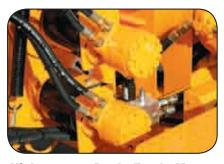
**High-torque Dual Feed Motors** provide the most infeed power of any 6" capacity chipper. These feed motors are rated for pressures higher than they are used at, which maximizes life.
