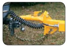
**Adjustable Height Hitch** easily adjusts to different tow vehicles to keep the chipper level and aid in safe towing.
