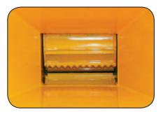
**10** ½" **Diameter Feed Roller** aggressively pulls in the material to be chipped. This extra large diameter feed roller climbs over material easily, pulling it into the chipper with no assistance. The high torque bottom roller aids in the feeding.
