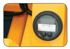
**Digitally Controlled Autofeed** monitors engine rpm and stops the feed automatically. This system has the ability to start and stop the feed of material into the chipper based on parameters set by the operator.
