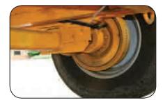
10,000-pound Capacity Dexter **Torflex Axle** makes the 2518 tow great, while minimizing turf damage.
