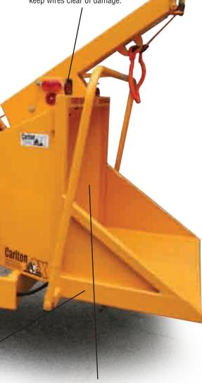
Massive 25" x 18" Throat Opening is the largest in its class and easily handles the largest tops.
