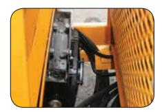
**Integrated Hydraulic Cooler** is tucked out of harm's way. Reduces fluid temperatures, increasing performance and extending component life.
