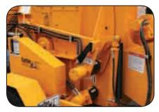
**Long Arm Pivot Design** allows the feed wheel to easily open over the largest butt ends. Frame extends beneath the infeed table for the ultimate in strength.
