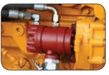
Tandem Pump System provides power independently to each feed wheel. This system ensures the most power at all times to the feed system.
