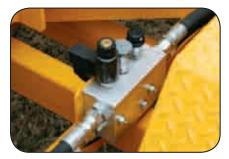
**Integrated Single Manifold Hydraulic System** simplifies the system reducing the number of hoses needed and reduces leak points. Variable feed speed control is standard on the 1712.
