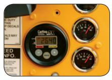
**Digitally Controlled Autofeed** monitors engine RPM and adjusts the feed automatically. This system has the ability to start and stop the feed of material into the chipper based on parameters set by the operator.
