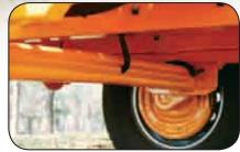
**7,000 lb. Dexter Torflex Axle** with Electric Brake makes the 1712 tow great.
