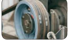
**Kevlar Construction Belts** carry more horsepower with less stretch, lowering maintenance costs and prolonging belt life.
