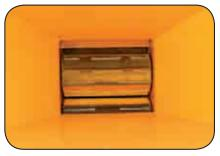
**101/2" Diameter Feed Rollers** aggressively pull in the material to be chipped. These large diameter feed rollers climb over material easily, pulling it into the chipper with no assistance.
