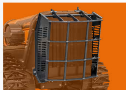
Steel radiator protection
