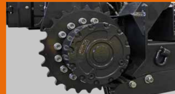
Cogwheel of the tracks in tempered steel
