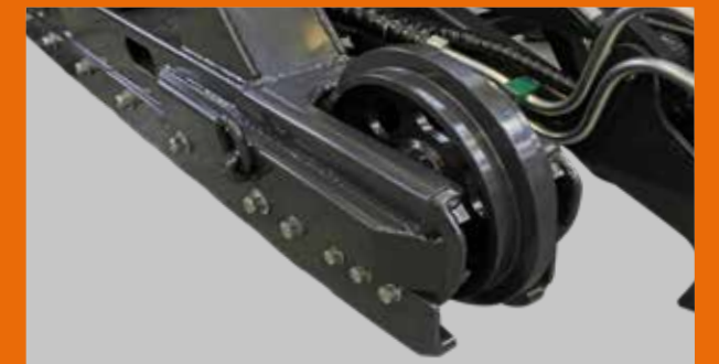
Track tensioner with safety spring
