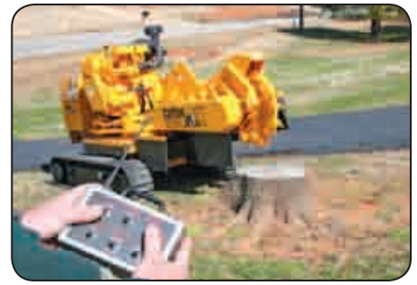
Wireless Remote Control keeps the operator out of the dust, debris and noise.
