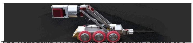
The voyager HD Mainline Inspection System is a high definition video system for inspecting mainlines relined 6" - 48" and up. The complete system includes a powerful transporter, a full HD 1080p WiperCam camera, and 1200' cable reel controlled by CANbus technology for instant
