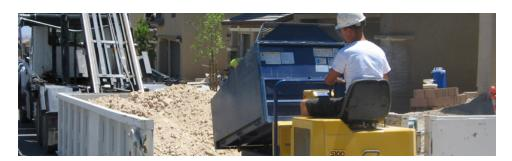
The Canycom S100 Compact Carrier with 180° Pivoting Dump Box is designed for excellent performance and maneuverability in extreme conditions. At only 39 inches wide, the S100 is perfect for fitting in narrow spaces. The 15 HP Kubota Diesel engine hauls up to 2,210 LBS and climbs grades up to 25° with ease.
