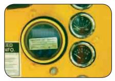
**Digitally Controlled Reversing Autofeed Plus** monitors engine rpm and adjusts the feed automatically. This system has the ability to start, stop, and reverse the feed of material into the chipper based on parameters set by the operator.
