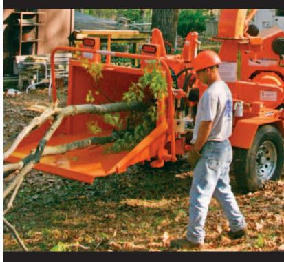
The Carlton 1790 wood chipper is built to withstand the punishment you dish out. From the heavy duty infeeders to the formed infeed, the Carlton 1790 is the most solidly constructed chipper on the market today. Thoughtful design elements like concealed wiring and full-length radiator protection guards keep the 1790 operating at peak performance from year to year. For **DURABILITY** and **DEPENDABILITY** nothing compares to Carlton.
