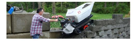
Canycom's newest additions to our concrete line allows contractors to access narrow sites unimaginable with other machines. Rubber tracks and an overall width of 29" inches allows operators to pass through garden gates, climb steep slopes, and work in the tightest and roughest of worksites.
