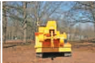
Carlton's patented turret bearing design provides the Hurricane TRX with 360-degree continuous rotation. This gives the Hurricane TRX massive cutting dimensions, allowing the machine to cut a full 19-foot width.
