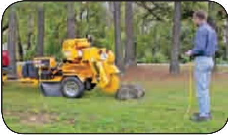
Optional Wired Remote distances the operator from dust, noise and flying debris.
