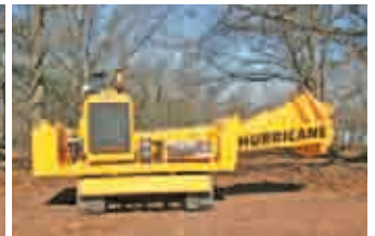
Carlton's patented turret bearing design provides the Hurricane TRX with 360-degree continuous rotation. This gives the Hurricane TRX massive cutting dimensions, allowing the machine to cut a full 19-foot width.
