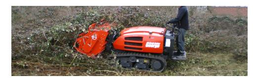
The CG431 is a heavy duty rubber track brush cutter designed to trim tough, overgrown brush on slopes, uneven, unstable ground, and areas with hard to reach ledges such as riverbeds. Smooth hydrostatic transmission for precise maneuverability.
