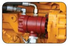
**Tandem Pump System** provides power independently to each feed wheel. This system ensures the most power at all times to the feed system.
