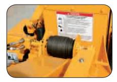
**Hydraulic Winch** will accept cable or rope. Winch includes freewheel capability.
