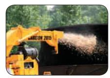
**Carlton's Exclusive Air Vortex Control** channels and accelerates discharge air giving the Apache series high discharge velocities and great chip throwing power.
