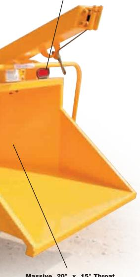
Massive 20" x 15" Throat Opening is the largest in its class and easily handles the largest tops.
