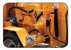
The Combination of Three Hydraulic Feed Motors, Carlton's exclusive long arm pivot, and the oversized 15¾" top feed roller give the 2015 the best feeding characteristics available.
