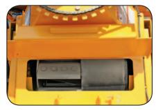
**Dual Edge Knives** are easily accessible, making routine maintenance an easy process. Bolts and Nuts are both removable eliminating problems caused by cross threading or stripping pockets.
