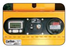
**Digitally Controlled Reversing Autofeed** monitors engine rpm and adjusts the feed automatically. This system has the ability to start, stop, and reverse the feed of the material into the chipper based on parameters set by the operator.
