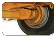
**10,000-pound Capacity Dexter Torflex Axle** makes the 2015 tow great, while minimizing turf damage.
