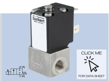
Type 2871 direct-acting proportional solenoid control valves are used as the regulating unit in control loops. Precise control is provided by utilizing Burkert's proportional control technology, a Type 8605 PWM Digital Controller.
