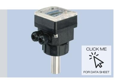
With a stainless steel insertion finger and high quality electronic display module this unit is perfect for contaminated or aggressive fluids. 4-20 mA and pulse output with optional 3A relays makes this a flexible solution for flow control, batching or CIP control in FDA applications.
