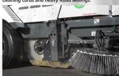
**DUST SUPPRESSION SYSTEM** • Global M4 includes 250-Gallon Water Tank Capacity combined with Two(2) Diaphragm Water pumps and Two(2) Modes (LOW/HIGH) provide versatility and superb dust control.
