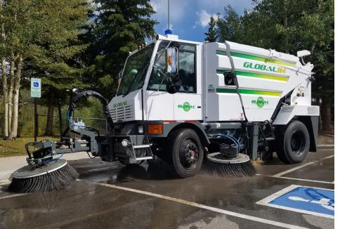
THREE POWERFUL BROOMS Optional Front Articulating brush allows for extra reach to shoulders and center islands Via In-cab joystick, the articulating front brush can be positioned on left or right side allowing for sweeping on right or left without changing seating positions.
