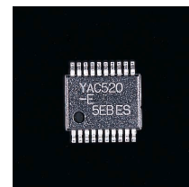
Digitally Regulated Volume Control Device (Yamaha Original YAC-520 LSI)
