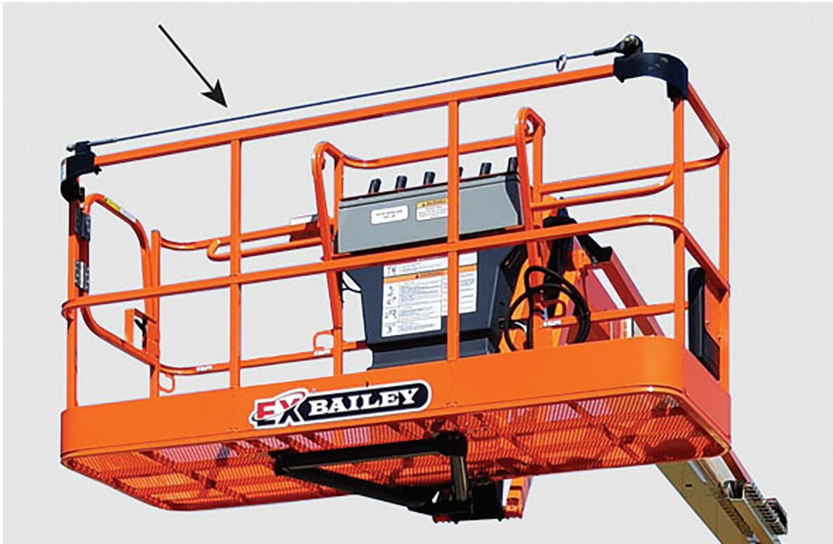
A Bolt-On Fall Arrest System can be bolted to existing JLG platforms in the field.
