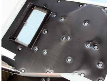
SILENT PLUS PACKAGE QUIET SWEEPING OPERATION The "Silent Plus" option utilizes sound supressive material in the engine compartment effectively reducing noise pollution during sweeping to 87 dB(A).
