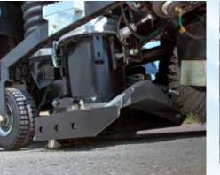
THE "V-NOZZLE" WILL SWEEP IT ALL The V-shaped Suction Nozzle with its large aperture, made of 4mm steel, conveys the swept material directly into the suction tube. This design enables the **Global V6AIR** to lift the Heaviest of debris in any application.
