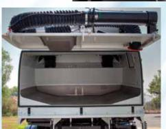
QUALITY, BUILT TO LAST STAINLESS STEEL CONSTRUC- The Global V6AIR includes Galvanized Hopper Screens that TION Hopper Design includes only the best such as 304 Grade Stainless Steel (100%) integrated into the 8.5 Cu.Yd. Hopper
