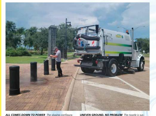
ALL COMES DOWN TO POWER The sloping configuration of the suction fan optimizes the air flow and increases the suction power while reducing wear.
