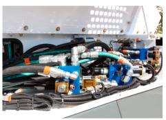
IT'S ALL IN THE OPEN Hydraulic Hoses are NOT hidden in the frame of the sweeper, while all Manifolds and Filters located in a central location.
