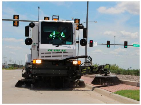
**THREE POWERFUL BROOMS Optional** Front Articulating brush allows for extra reach to shoulders and center islands. Via In-cab joystick, the articulating front brush can be positioned on left or right side allowing for sweeping on right or left without changing seating positions.
