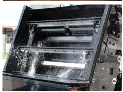
HEAVY SWEEP PACKAGE Elevator Type: Standard 11 Flight squeegee with replaceable corded rubber tips; Continuous molded rubber belts combined with standard Heavy Sweep Package make Global M3 CNG the logical choice for sweeping heavy debris such as road millings, sand and gravel up to 3-tons per-minute. That is one ton of sand every 20 seconds! Standard leaf gate system assists in picking up large debris, bottles, large branches and leaves.
