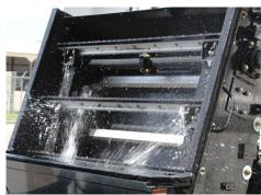
**HEAVY SWEEP PACKAGE** Elevator Type: Standard 11 Flight squeegee with replaceable corded rubber tips; Continuous molded rubber belts combine with standard Heavy Sweep Package make **Global M4** CNG the logical choice for sweeping heavy debris such as road millings, sand and gravel up to **3-tons per-minute**. That Is one ton of sand every 20 seconds! Standard leaf gate system assists in picking up large debris, bottles, large branches and leaves.
