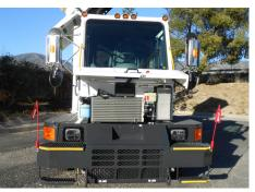
ACCESS IT ALL The Global M4 CNG features many maintenance-friendly attributes, such as a rear swing-out radiator, easy access front mounted AC condenser, brake and windshield washer fluid reservoirs, and cab fresh air filter
