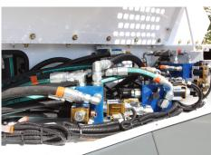
IT'S ALL IN THE OPEN Hydraulic Hoses are NOT hidden in the frame of the sweeper, while all Manifolds and Filters
