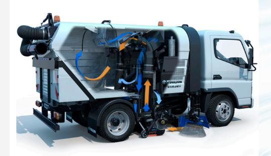
"Patented Sweeping System" Our Air Recirculation Technology (VAST) allows for sweeping below freezing conditions while expelling 50% less fine dust emission compared to a pure vacuum concept.
