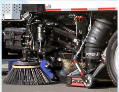
**THE POWER BRUSH** The channel brush or main transfer broom is mounted as a trailed brush and suspended separately from the suction nozzle. It is equipped with lateral shock absorbers and ground pressure adjustment in order to pick up heavy dirt off the road surface. The pneumatically controlled adjustment of the main transfer broom offers the best possible performance in every working condition.
