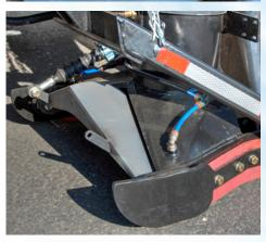
**THE "V-NOZZLE" WILL SWEEP IT ALL** The V-shaped Suction Nozzle with its large aperture, made of 4mm steel, conveys the swept material directly into the suction tube. This design enables the **Global V4AIR** to lift the Heaviest of debris in any application.
