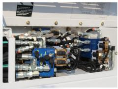
IT'S ALL IN THE OPEN Hydraulic Hoses are NOT hidden in the frame of the sweeper, while all Manifolds and Filters are located in a central location.
