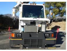
ACCESS IT ALL The Global M4HSD features many maintenance-friendly attributes, such as a rear swing-out radiator, easy access front mounted AC condenser, brake and windshield washer fluid reservoirs, and cab fresh air filter.
