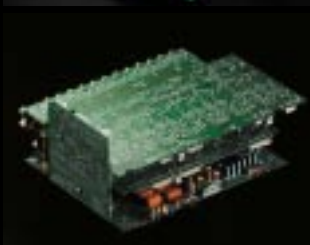
Preamplifier circuit board (top) and printed circuit board (bottom).
