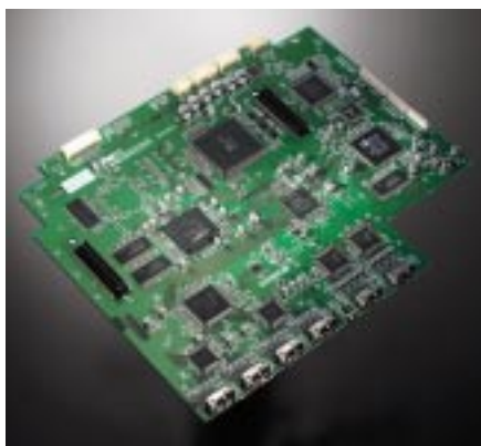
Digital video circuit board (left) and analog video board (right).
