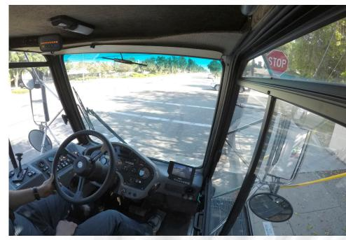
THE BEST TURNING RADIUS & EXCEPTIONAL VISIBILITY With the center mounted cab/forward layout the operator has unsurpassed visibility of the road surface as well as pedestrians and surrounding traffic. The 130-inch wheelbase allows for the sweeper to reach a turning radius of 18 1/2', wall-to-wall. With the pickup Head in the center you don't have to worry about what is happening behind you. The Global R4AIR EV's exceptional visibility increases operator and pedestrian safety.
