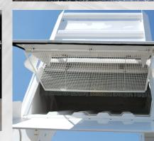
LARGEST HOPPER IN IT'S CLASS Global R4AIR EV includes a 5.8 cu/yd 100% Stainless Steel hopper construction, Cyclone Type Dust Separators and Swing-Down Hopper Screens are easy to clean.
