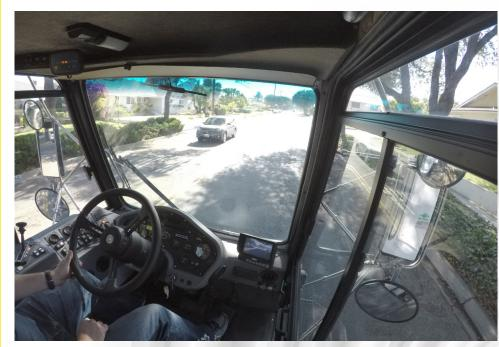
The inherent design of the Global M3EV makes it the only choice among 3-wheel mechanical sweepers. With the center mounted/cab forward layout the operator has unsurpassed visibility of the road surface as well as pedestrians and surrounding traffic. The large hopper capacity equals more lane miles swept between dump cycles and the 12.5-foot turning radius makes the Global M3EV highly efficient and comfortable.
