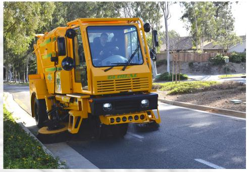
With travel speed of 25-MPH and a battery operational range of 9-11 hours, towns, villages and large cities will be able to clean the streets while protecting our environment and building a cleaner future with ZERO EMISSIONS. At the end of the shift just plug in the sweeper, recharge the batteries and sweep again
