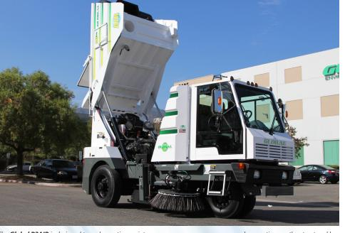
The Global R3AIR is designed to make routine maintenance easy, so your sweeper spends more time on the street and less time in the garage. Two swing-out center body panels provide unrestricted access to Fan Housing, maintenance and daily cleaning. A centralized, weather-proof systems locker fully protects electrical components from the elements while fender located Hydraulic system allows for easy maintenance, accessibility and inspection. Troubleshooting is now a breeze
