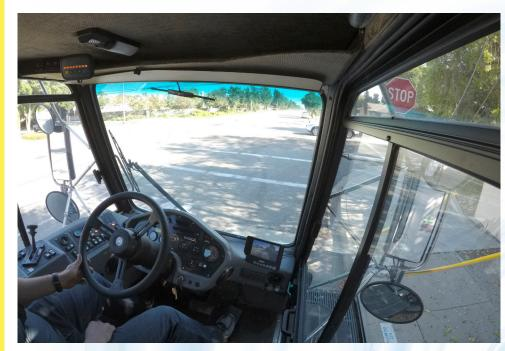
THE BEST TURNING RADIUS & EXCEPTIONAL VISIBILITY With the center mounted cab/forward layout the operator has unsurpassed visibility of the road surface as well as pedestrians and surrounding traffic. The 116-inch wheelbase allows for the sweeper to reach a turning radius of 12 1/2', wall-to-wall. With the pickup Head in the center you don't have to worry about what is happening behind you. The Global R3AIR's exceptional visibility increases operator and pedestrian safety.
