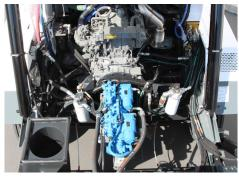
The **Global R3AIR** comes standard with a fuel-efficient Final T4 4-cylinder, turbocharged 172-horsepower Isuzu diesel engine, largest in its class, delivering outstanding performance and reliability.
