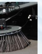
**POWERFUL GUTTERBROOMS** Large 47" Digger-Type Gutterbrooms allow for
