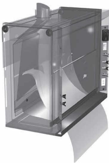
VAV Fume Hood Sash Closed
