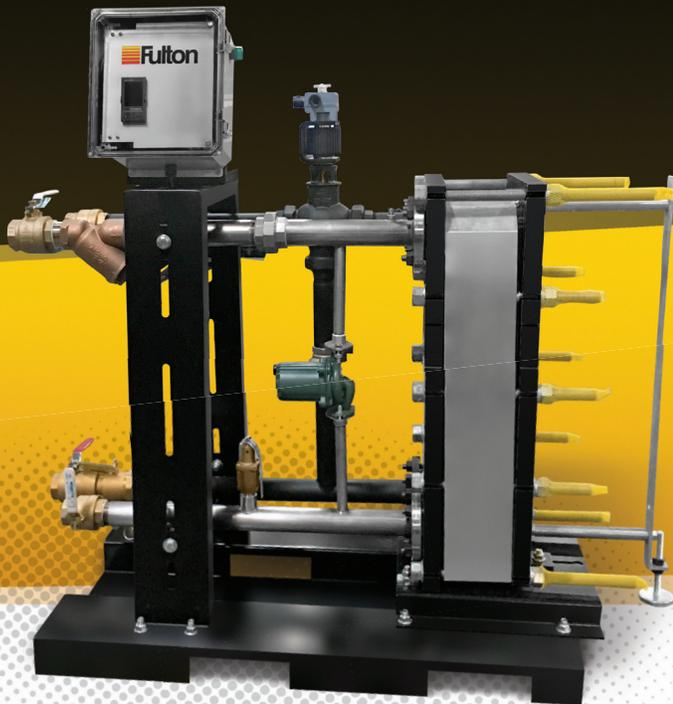
The InTherm Series indirect water heaters deliver up to 90 GPM of hot water using high-efficiency plate-and-frame heat exchangers with real-time load tracking, eliminating the need for large storage tanks. Designed for compact spaces, they offer easy maintenance with removable heat exchangers, isolation valves, and backflush connections.
