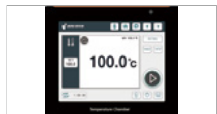
Controller for temperature. (TC3-model)
