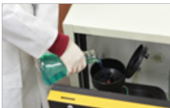
Wide inlet of waste liquid funnel.
