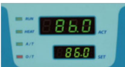
Simultaneously displays set temperature and actual temperature.
