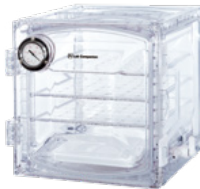
VDC-31 (Cubic type) with Vacuum Gauge (standard)
