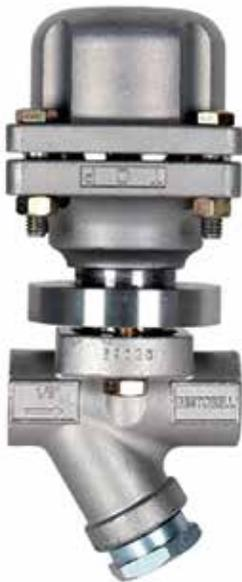
The Universal Trap is a bimetallic steam trap for plant applications requiring standardized connections. The mounting connections allow trap use on any manufacturer's universal mount. The two bolt replacement module allows for ease in installation and replacement. A built-in check valve prevents back flow. It automatically adjusts to operating pressure and load changes, overcoming problems associated with cycle discharge.
