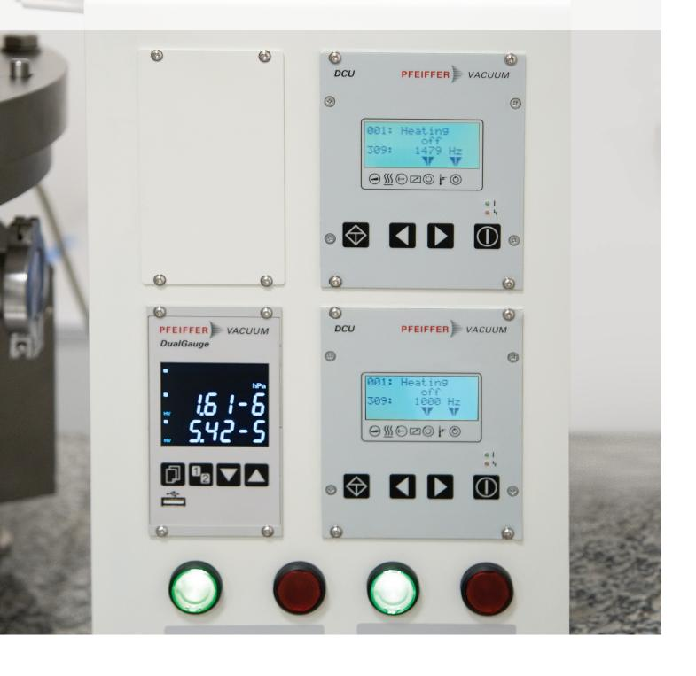
Controller set for operation of preliminary and turbomolecular pump of the main chamber and LOAD LOCK system, and vacuum gauge controller.
