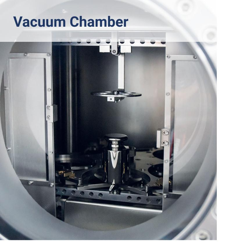
Used chamber enables comparison in vacuum of maximum  $10^{(-6)}$  mBar or in noble gases such as argon.
