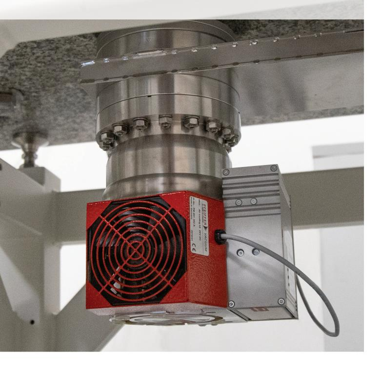
Turbomolecular pump used to maintain vacuum at the level of  $10^{(-6)}$  mBar.
