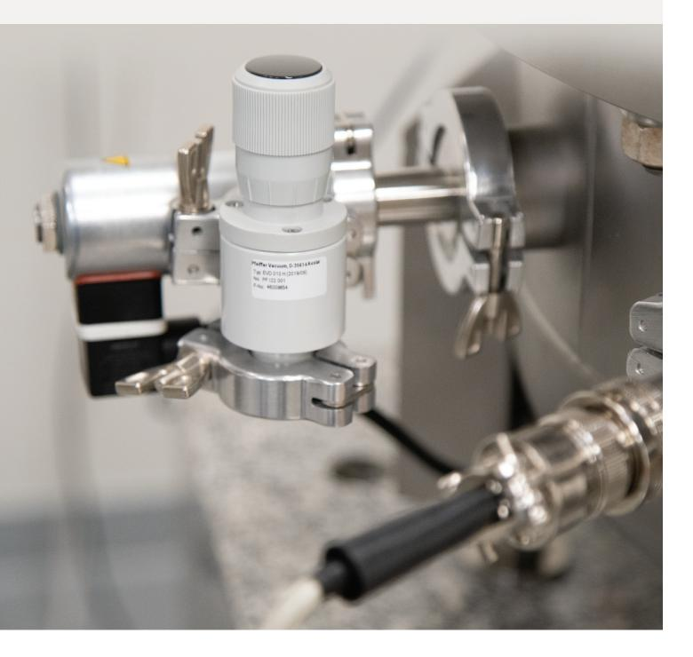
The main chamber of mass comparator is equipped with 8 flanges (DN 40 ISO KF) for connecting devices such as vacuum gauge, solenoid valves, CO<sub>2</sub> sensors, etc. LOAD LOCK chamber features 2 such flanges.
