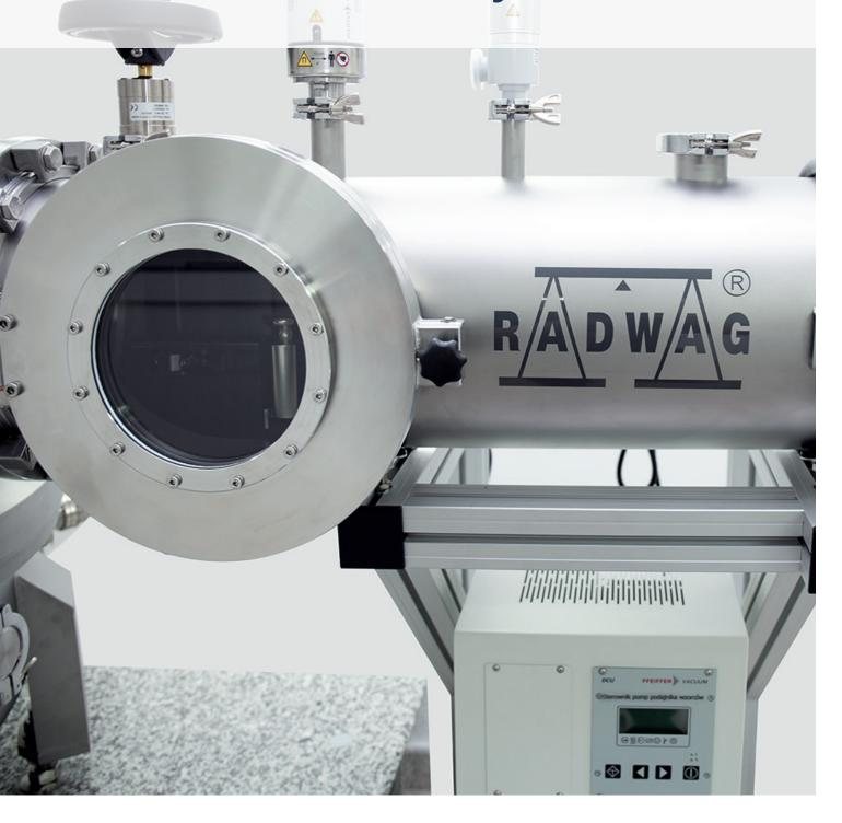
The LOAD LOCK system for transfer of mass standards enables switching and adding artefacts without changing the atmosphere inside the main chamber.
