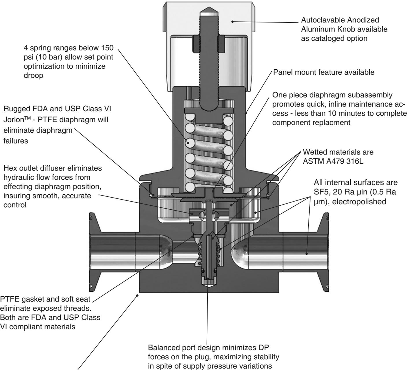
**NOTE:** Can be used on clean steam or non-cavitating liquids (the design is not drainable) with Steriflow engineering application approval.
