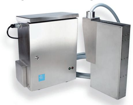
The Filtrax and Filtrax eco Sample Filtration Systems continually extract samples directly from process effluent and pull the water through ultra-filtration membranes (0.15  $\mu$ m) that are immersed in the aeration basin or primary settling tank.
