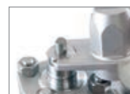
Tightening the gland retainer
