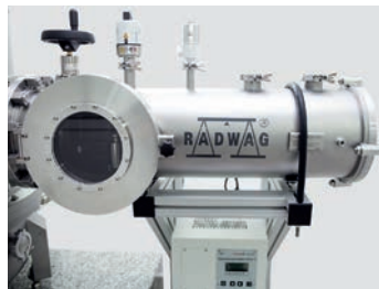
The LOAD LOCK system for transfer of mass standards enables switching and adding artefacts without changing the atmosphere inside the main chamber.
