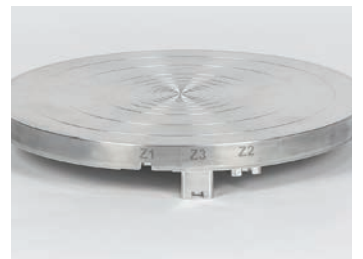
Specially designed susceptometer weighing pan does not require any additional elements to change the measuring range of the device.
