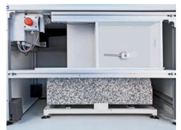
Sturdy design of the table, featuring heavy granite stone and robust rubber shock absorbers, reduces effect of vibrations to the absolute minimum.
