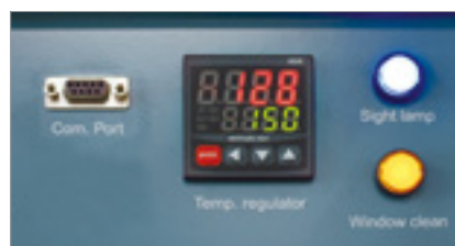
Electronic over temperature protection system.
