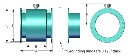
Dura Mag meters are available in lay lengths compatible with products from other meter suppliers. See the tables below for matched lay length options.
