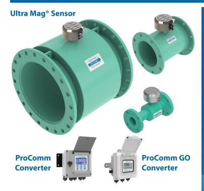
Ultra Mag flow meters are manufactured to the highest standard available for mag meters. The flanged end tube design permits use in a wide range of applications with up to 300 PSI working pressure. The fabricated tube is stainless steel with steel or stainless steel flanges and is lined with UltraLiner™, an NSF approved, fusion bonded epoxy material.
