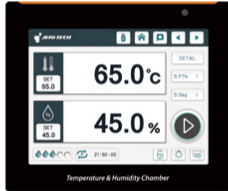
Color touch display controller (5.6 inches)
